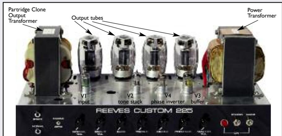
Fig. A Front row (left to right): V1 - NOS Baldwin 12AX7; V2 – new Tung Sol 12AX7; V4 – NOS GE 12AT7; V3 – new Electro Harmonix 12AX7; Back row: four new JJ KT-88’s
