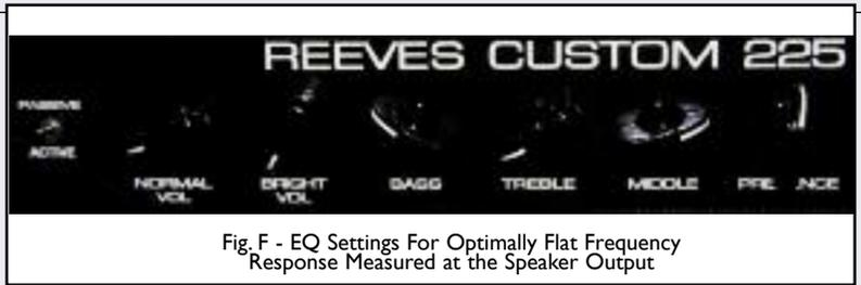
Fig. F - EQ Settings For Optimally Flat Frequency Response Measured at the Speaker Output
